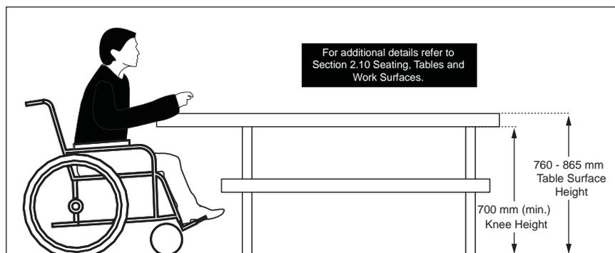
**Figure 96b:** Picnic Table Design and Features - Elevation View
