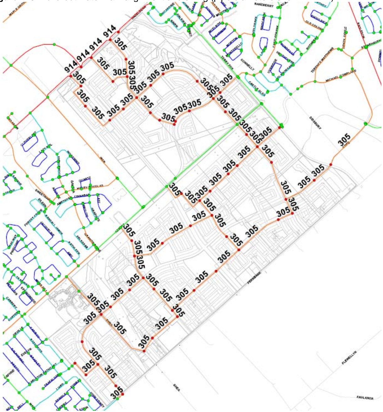
Figure A-5: Build-out watermain alignment and sizing (pipe diameters shown in mm)
