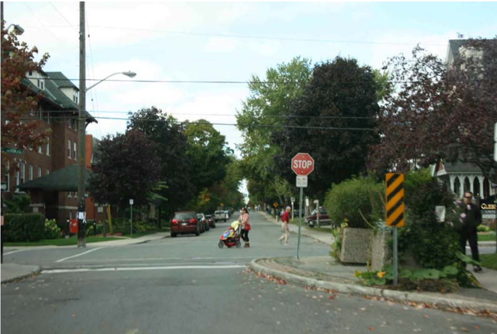
The vegetation planters installed at this Ottawa intersection can easily obscure the driver's view of a pedestrian waiting to cross the street. Can you see the pedestrian on the sidewalk on the right side of the photo? (McCormick Rankin Corporation)
