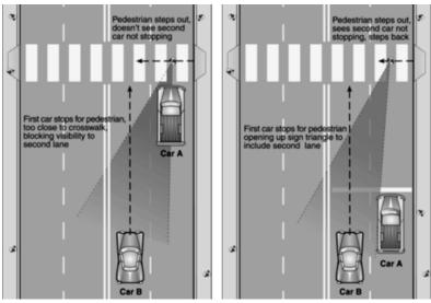
This diagram illustrates the improvement in visibility between drivers and pedestrians that can be attained when vehicles stop further back from the crosswalk. The increased space also creates a buffer between vehicles and pedestrians. (www.walkinginfo.org)
