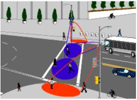
Microwave or a similar technology detect the presence of pedestrians waiting and crossing the crosswalk, eliminating the need for a push-button and sometimes adjusting signal timing if necessary (www.walkinginfo.org / ITS Technologies)
