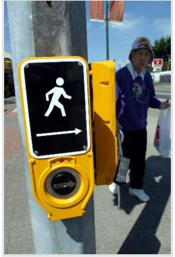
The above APS push-button is one example of the many types that provide a locator tone to help visually impaired pedestrians find it and provides audio and vibrotactile feedback corresponding to the "walk" indication in the crossing direction indicated by the tactile arrow. (www.pedbikeimages.org / Dan Burden)
