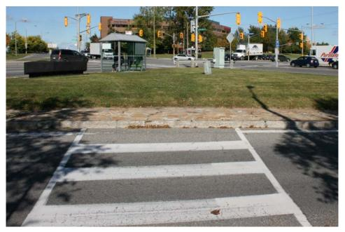
In this photo, a crosswalk is provided across a channelized right turn lane at the Baseline / Prince of Wales intersection. At this location there is no curb ramp, a very rough texturized sidewalk treatment not conducive to mobilibity challenged or pedestrians requiring assistive devices, and a very limited refuge area. These types of conditions present significant challenges for pedestrians. (McCormick Rankin Corporation)
