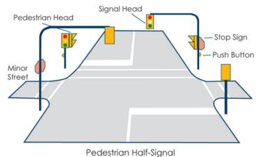
Half-signals interrupt major street traffic only when activated by a pedestrian push-button. A typical configuration is shown above. (Halifax Regional Municipality)
