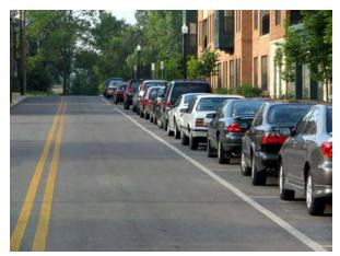
An example of on-street parking. It provides a buffer between traffic and pedestrians and narrows the roadway—helping to reduce vehicle speeds. However, on-street parking can limit the visibility of pedestrians. (www.pedbikeimages.org/ Dan Burden)
