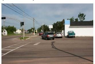
An example of poor access management adjacent to a crosswalk. In this case, there is no pedestrian refuge at the end of the crosswalk and vehicles make high speed movements in and out of the parking area. (McCormick Rankin Corporation)
