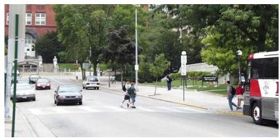
An example of a transit stop located on the near side of a crosswalk. Far side transit stops are generally safer from a pedestrian's perspective due to better visibility between pedestrians and drivers. (www.pedbikeimages.org / Dan Burden)
