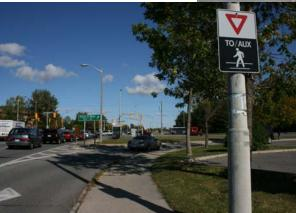
In the example above a sign blocks the driver's ability to see pedestrians crossing at the crosswalk. The example at left illustrates the sightline limitations to the crosswalk due to vegetation. Both of these obstacles are located at the same crosswalk and are relatively inexpensive to remedy. (McCormick Rankin Corporation)
